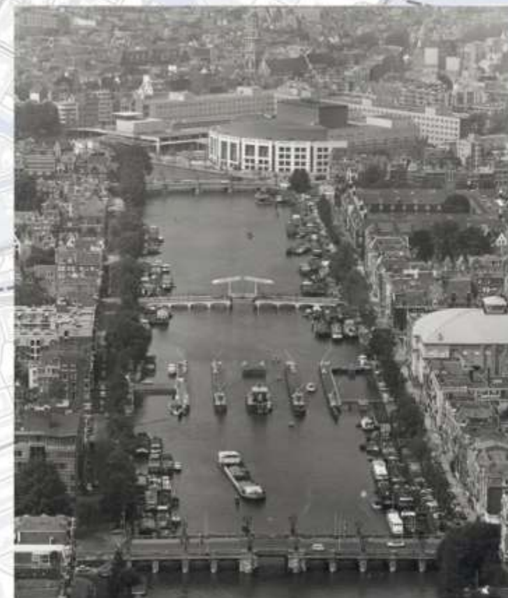
Blauwbrug, Magere Brug, Amstelsluisen and Hogesluis, crossing the Amstel river and regulating the water level.
